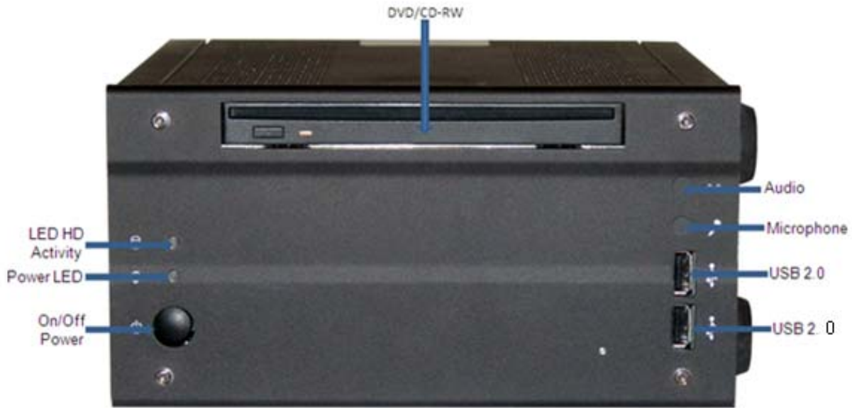
Figure 5-3 SV-100 M-DVR Components and Connectors (Front View)
